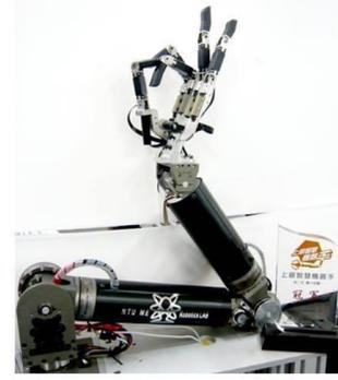
Fig. 3. 6-DOF NTU robot arm.
