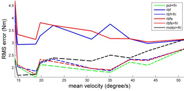
Fig. 5. RMS error of torque prediction in experiments, evaluated on the remaining 2/3 of collected data.
