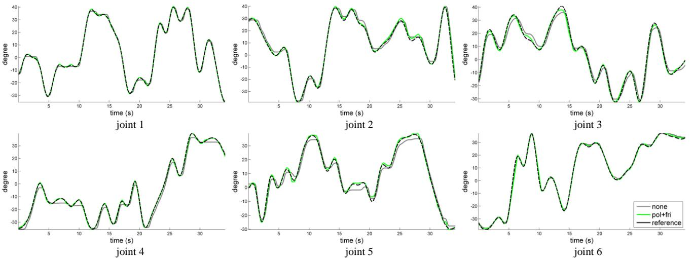
Fig. 8. The results of tracking a joint-space trajectory that transverses through randomly selected points over the workspace (*none* denotes PD position feedback alone).
