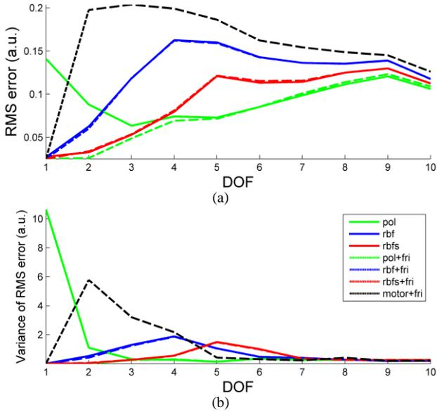
Fig. 2. RMS error of prediction in learning the ideal model with simulated friction and Gaussian measurement noise. (a) mean (b) variance.
