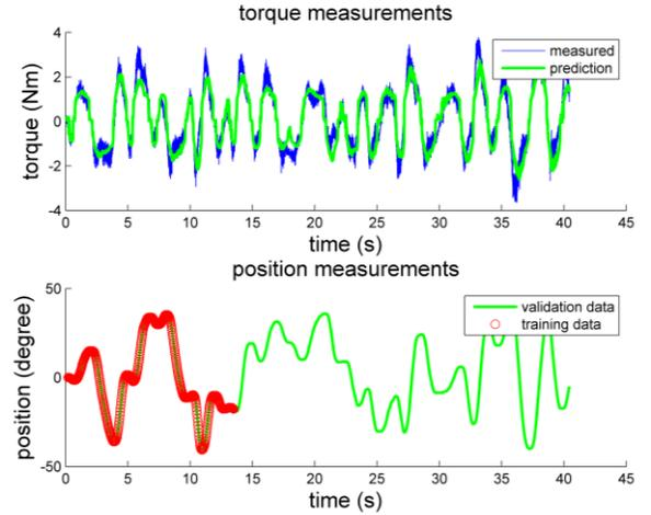
Fig. 4. The collected data and the prediction of *pol+fri* of joint 3. Each model is trained with the first 1/3 of the collected data, and tested on the rest 2/3. The validation trajectories traverse the workspace with a speed gradually ascending.
