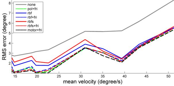
Fig. 6. RMS error of position trajectories in experiments, evaluated on the remaining 2/3 of collected data (*none* denotes PD position feedback alone).
