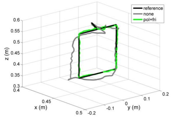
Fig. 7. The results of tracking a square trajectory (*none* denotes PD position feedback alone).
